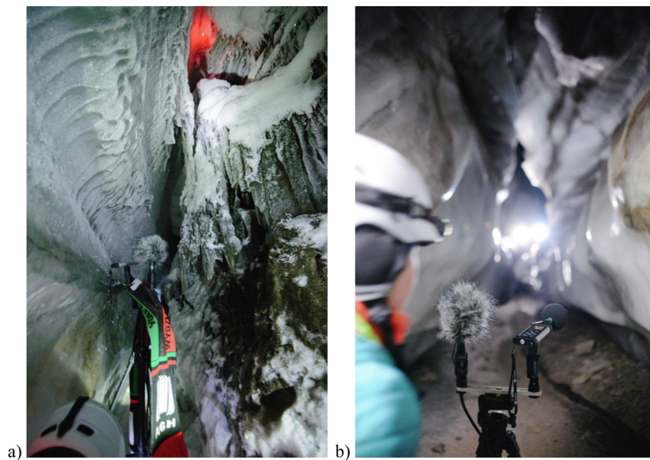
Fig. 5. a, b) Ambisonic microphone and sound pressure level meter in the studied cave corridors.
