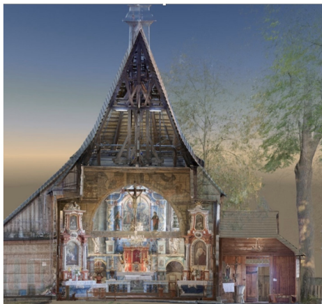
Fig. 2. Illustration of the laser scanning process and subsequent data postprocessing applied to the Church of All Saints in Blizne.
